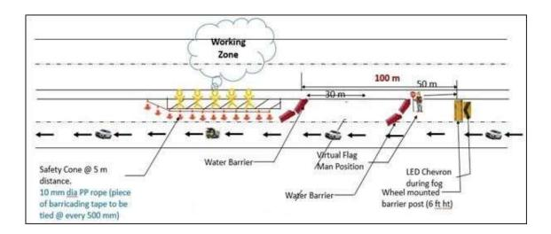
Note - In addition to the above "Men at Work" (900 mm) & Arrow marking should be placed on the live carriageway at least 500 m ahead of working place.
